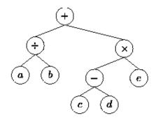
The terminal nodes (leaves) of an expression tree are the variables or constants in the expression (a, b, c, d, and e). The non-terminal nodes of an expression tree are the operators  $(+, -, \times, \text{ and } +)$
