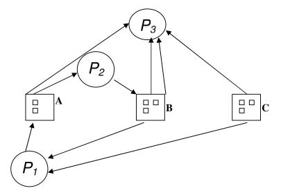
There is a cycle in the resource allocation graph implies system is not in a safe state. System is in deadlock as required resources are 1 unit of resource A and 1 unit of resource B while available resource is 1 unit of resource C. None of the process can be completed. Q.64 what is system programming? Explain the evolution of system software. (6)
