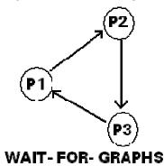
(ii) Periodically invokes an algorithm that searches for cycles in the graph. If there is a cycle in the wait-for-graph a dead lock is said to be exist in the system.
