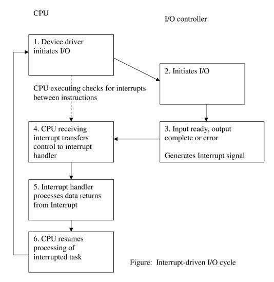
The CPU saves small amount of state, such as the current value of the instruction pointer i.e. return address, and jumps to the interrupt handler routine at fixed address in memory. The interrupt handler determines the cause of the interrupt, performs the necessary processing, and executes a return from interrupt instruction, thereby clearing the interrupt. The CPU resumes to the execution state prior to the interrupt.
