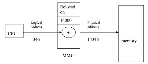
Mapping from logical to physical addresses using memory management unit (MMU) and relocation/base register
