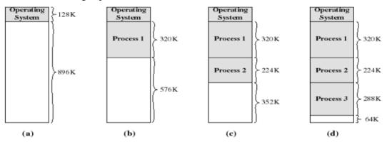
•A hole of 64K is left after loading 3 processes: not enough room for another process.
