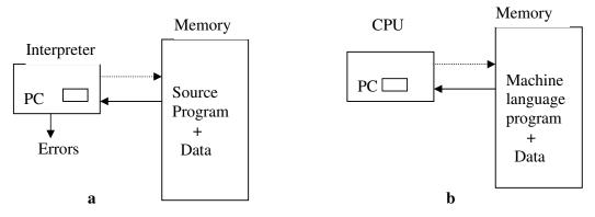
The CPU uses a program counter (PC) to note the address of next instruction to be executed. This instruction is subjected to the instruction execution cycle consisting of the following steps:
